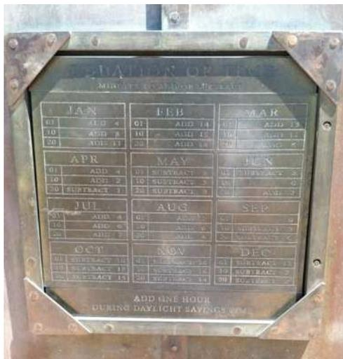
The 'key' below the sundial allows for addition or subtraction depending on the time of year to indicate accurate time.
