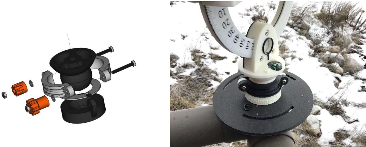
Figure: Circular Sundial Base on a Head-Leveling Ball Mounted on a Railing Post
