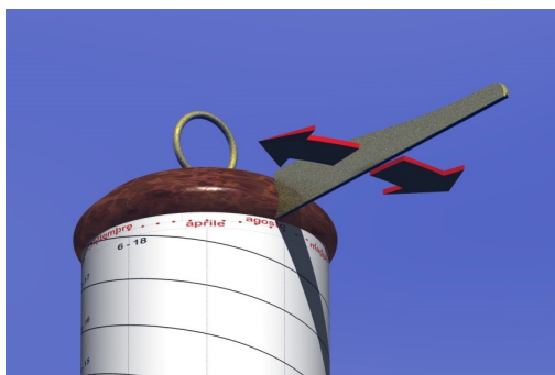
Fig. 6. Setting the gnomon position to match the declination of the Sun, by means of the calendar.
