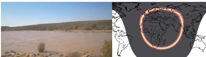
Fig. 30. (Left) Shadow of bush with lake in background. (Right) Given the UTC time and sun angle, the Bellingcat software creates a circle of altitude for the sun at that moment. Using local features (lake, road, building, etc.) Google Earth can help find the exact coordinates.
