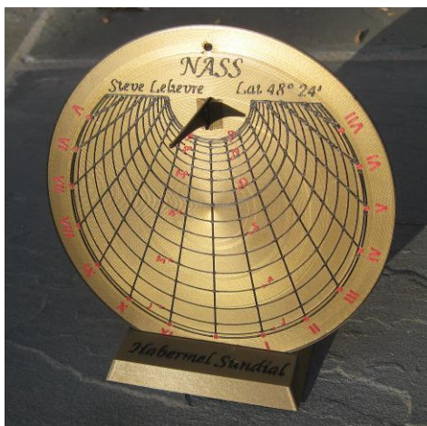
Fig. 35 Habermel dial made for Steve Lelievre at his latitude in Victoria, Canada.
