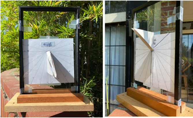
Fig. 31. Paul's experiment with a vertical semitransparent North/South Dial with gnomons on both sides.
