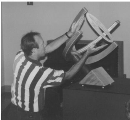
Pete Swanstrom described and showed his large Universal Equatorial Sundial with an analemmatic pierced plate gnomon. One version was constructed of wood, the other of brass. These indicate the time to the nearest minute, the date, and incorporate a quick adjustment for daylight savings time. He also discussed a similar stainless steel sundial for the Anne Morrison Park in Boise, Idaho. His talk and the very detailed written description of the design, fabrication, and
