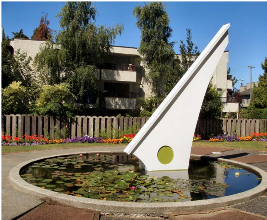
Buildings partially block the sun from this dial – only the lines for those hours and dates when the sun strikes the dial are marked on the ground.
