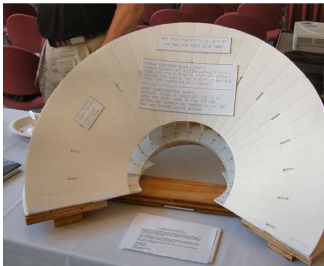
Chuck Nafziger's light concentration sundial, complete with Braille markings.
