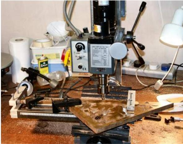
Fig. 5. Milling style edge on the waterjet-cut gnomon.
