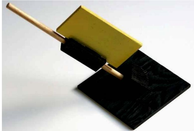
Figure 1 - polar rod with solar vane for 43°N at noon
