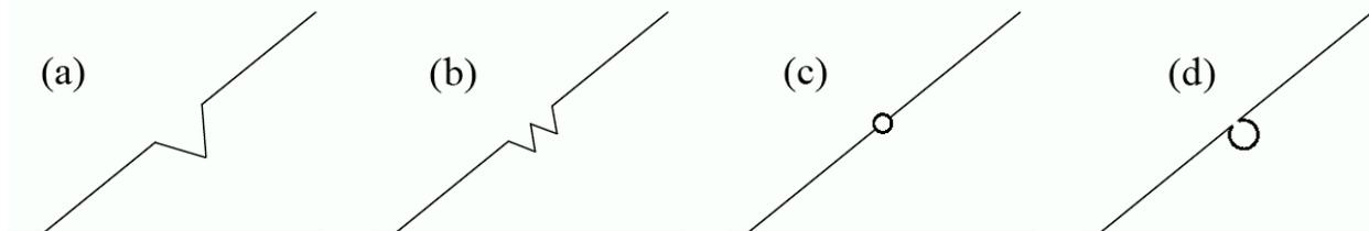
Fig. 4. Diagram of various nodus types for a horizontal dial. (a) V-cut, (b) ‘W’ form, (c) cross-cylinder, (d) through-hole.
