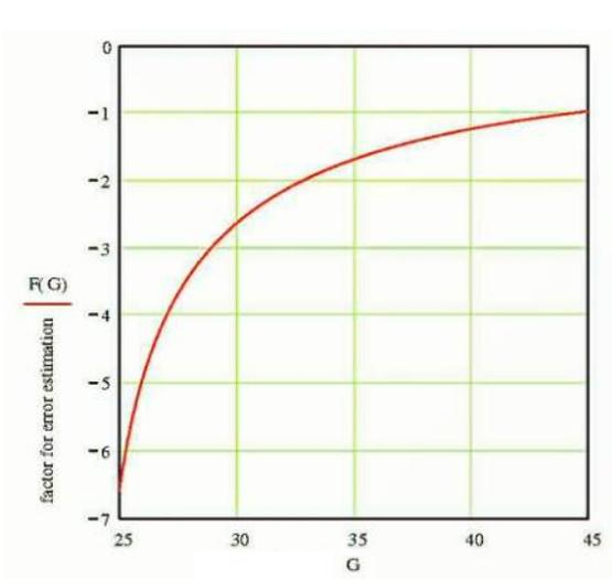
Fig. 2: Graphical representation of error estimation factor  $F$  from formula (19) depending on angle  $G$ ; sun's declination  $\delta_s = 23.4393^\circ$ .
