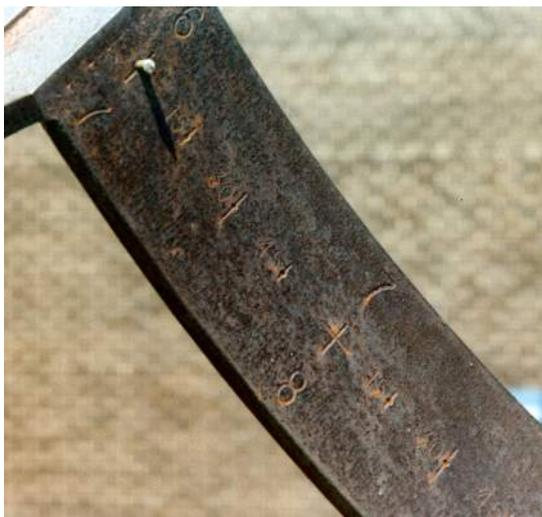
Equatorial arm, with hour lines (standard and daylight savings time). This also shows the attachment of the missing horizontal gnomon wire.
