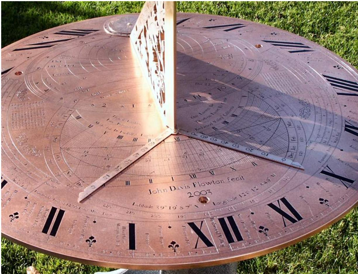
Fig. 9. The dial from the north, with the two alidades pivoted underneath the knife-edge.
