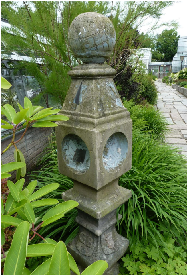
Fig. 17. The north faces of the Duthie Park dial with the wrong gnomons.
