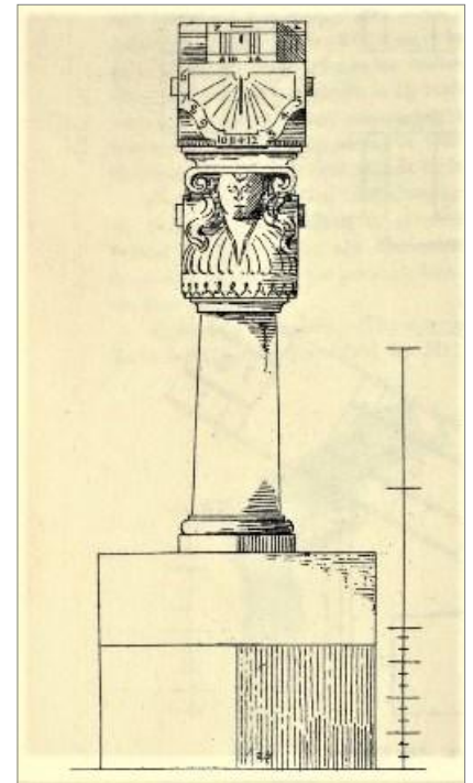
Fig. 7. Ross’s architectural drawing of the second Carberry dial.
