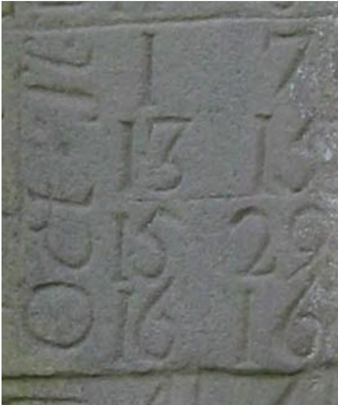
Fig. 10. Part of the EoT table for four dates in October (1, 7, 15 and 29). 'Oct' is written running upwards on the left of the block of eight numbers and the 'SC' which follows 'Oct' stands for 'Slower Clock'.
