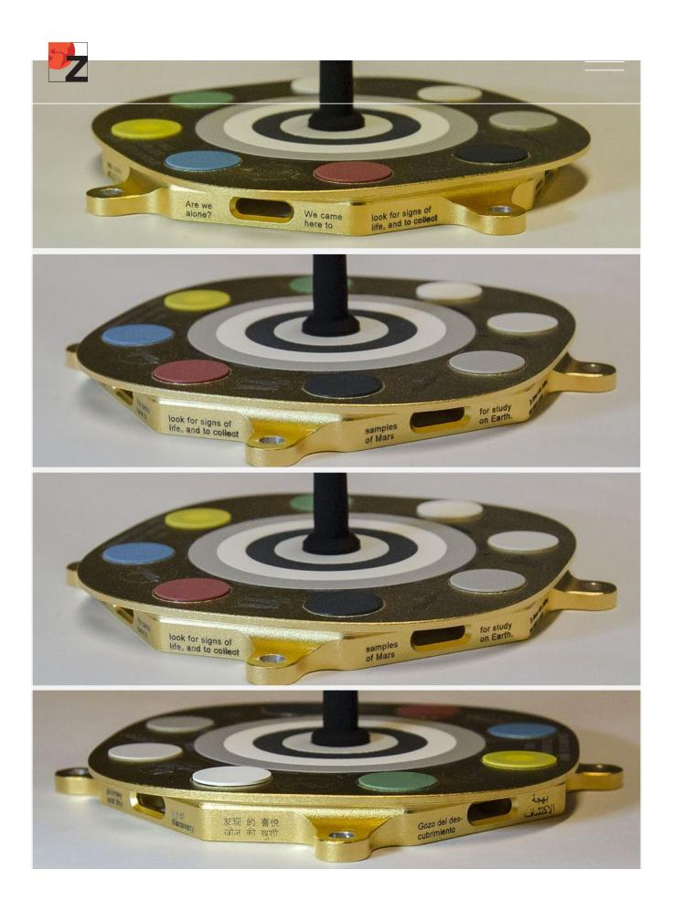
Figure 4: The "inspirational message" laser-engraved on the edges of the primary Mastcam-Z radiometric calibration target. Photo creates Bohr Institute, Copenhagen, Denmark/NASA/JPL-Caltech/ASU.
