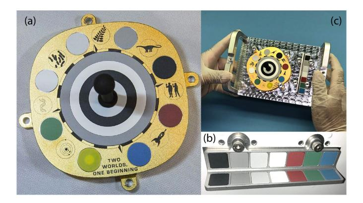
**Figure 1.** (a) The Mastcam-Z primary radiometric calibration target. The base of the target is  $\sim$ 9.8 x 9.8 cm (3.9 x 3.9 in); (b) The Mastcam-Z secondary radiometric calibration target. The length of the target is  $\sim$ 8 cm (3.1 in) and the "shelf" is  $\sim$ 1.6 cm (0.6 in) wide; (c) Inspection photo. Photo credits: (a) Niels Bohr Institute, Copenhagen, Denmark; (b, c) NASA/JPL-Caltech/ASU.
