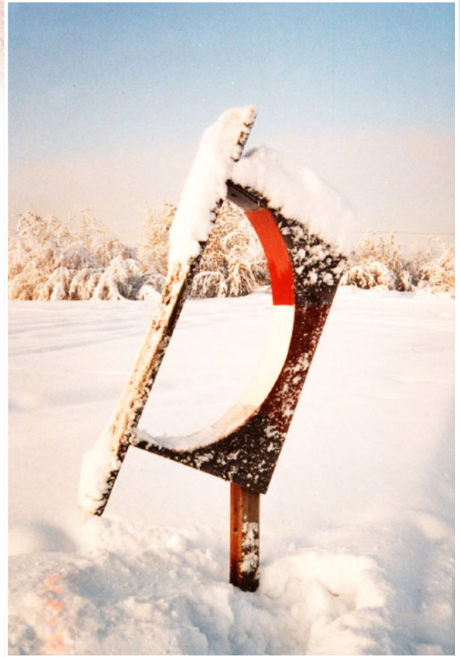
The full scale wooden mockup in winter installed at Weeks Field. The bottom of the painted red arc at the top face of the dial is where the sun's shadow should fall on winter solstice around December 21st when the sun reaches a maximum altitude of barely 1.5 degrees above the horizon.
