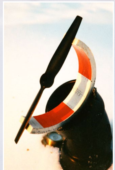
A 1/4" scale model was built from plastic sewer pipe and a model airplane propeller to test the sundial design at winter solstice.
