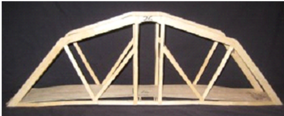
Fig. 4 Triangles add strength to a bridge.
