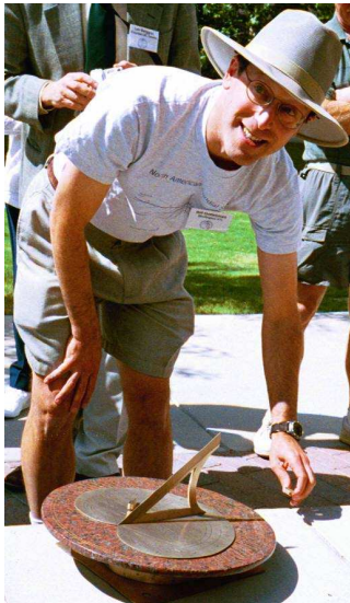
Here Bill Gottesman shows off his Sawyer Equant dial with the adjustments for latitude, longitude, equation of time and daylight savings time.
