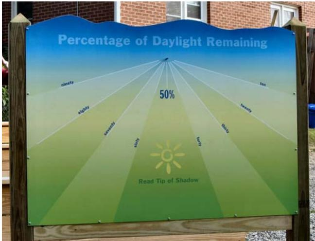
The dial is printed on a plastic coated aluminum sheet 1/8" thick and about 4ft. wide and 3ft. high, mounted on a wooden post and beam frame. This vertical dial faces due south so mid-day, 50% of daylight remaining is a vertical line straight down from the horizontal point gnomon. Again the reading is based on the shadow of the gnomon tip. The sun shines on the back or north facing side of the dial in the early morning and later evening during the spring and summer.
