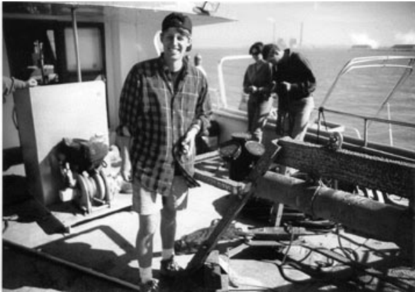
Mark Stacey BS '91 (Physics), MS '92, and Ph.D. '96 stands on the back of the USGS RV Turning Tide next to an ADCP (ours) that has recently been picked up after a two-month stay on the bottom of the Bay. The disk-like bodies on the ADCP head (near Mark's left hand) are the transducers themselves; these, thanks to Jeff Gartner's magic chile-vaseline preparation, are relatively free of encrusting organisms. The PG&E powerplant in Pittsburg can be seen in the background (Photo by J. Burau).
