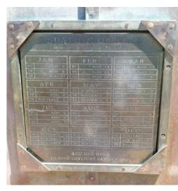
The 'key' below the sundial allows for addition or subtraction depending on the time of year to indicate accurate time.
