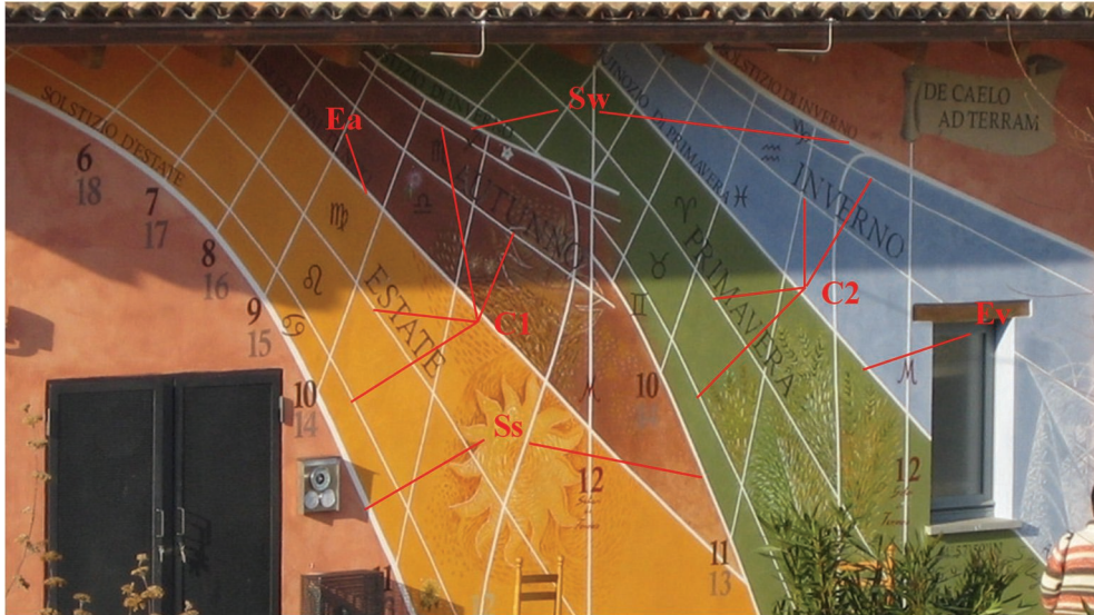
Fig. 6. The solstice, equinox and zodiacal month lines.
