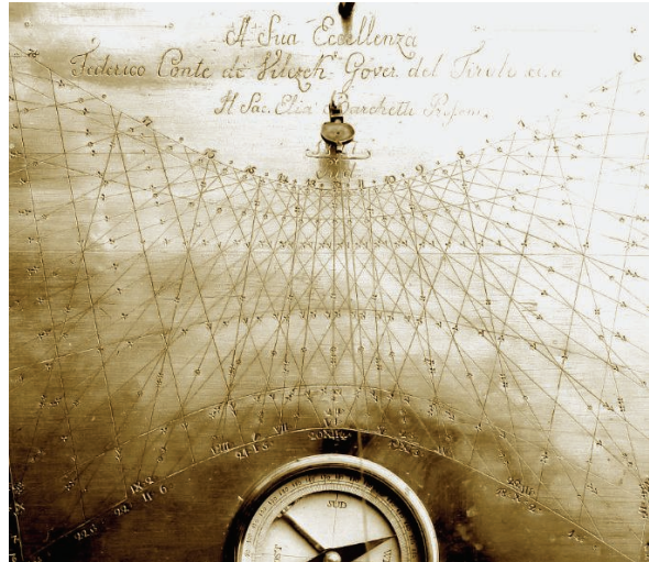
Fig. 2. The many lines of the Barchetti scale plate.
