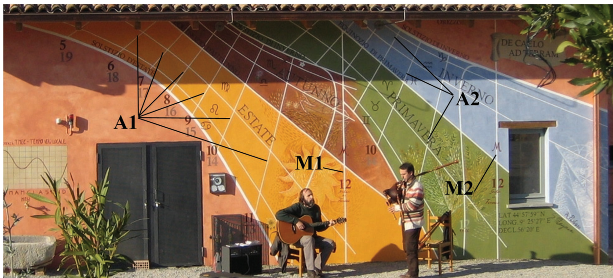
Fig. 2. The dial. M1 and M2 indicate the local meridians, apparent noon. Line sets A1 and A2 are other hour lines.
