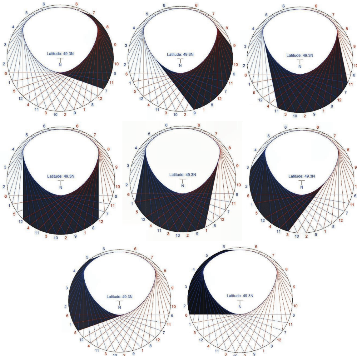
Figure 16. Throughout the day, the shadow intersects the same length arc on the hour circle. Time can be read from either edge of the shadow. Blue numerals, leading edge; Red numerals, trailing edge.
