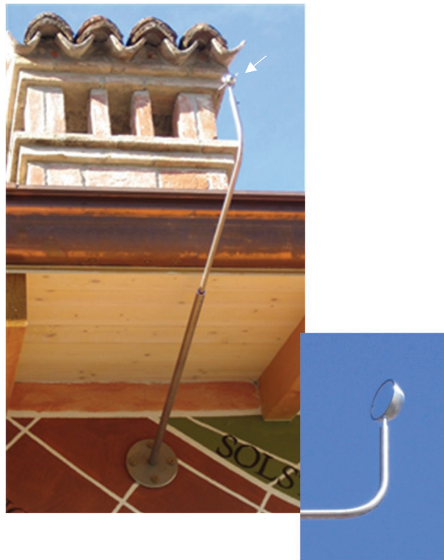
Fig. 7. The shadow caster / mirror combination and close view (inset).
