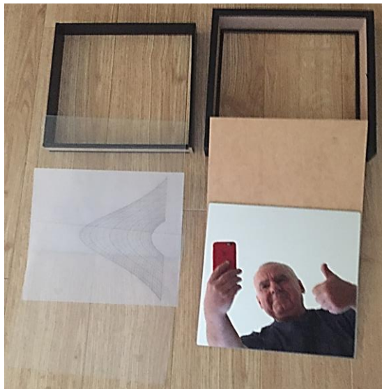
Fig. 4. Dial components. The transparent items, polycarbonate and glass, hardly visible in this photograph, are in the middle left and lower left.
