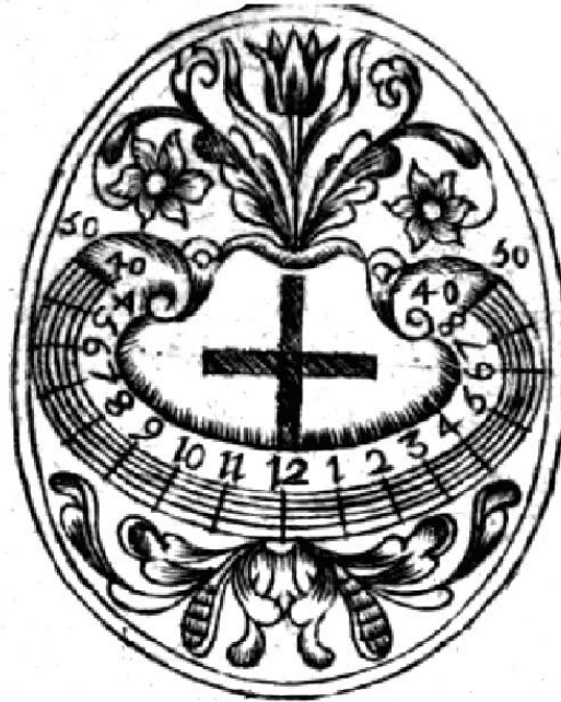
Top face of a universal George dial showing the elliptical hour lines and ellipse trammel cross.
