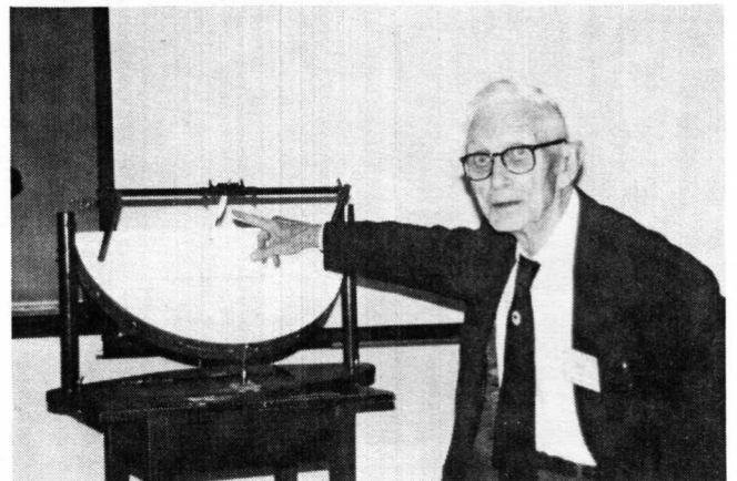
Bill Buckler demonstrates his analemmic gnomon on an equatorial dial.
